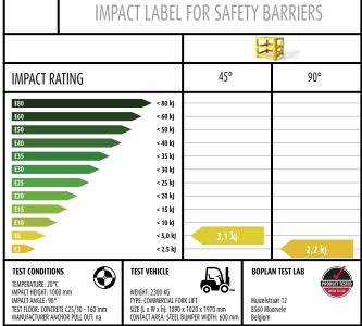
$\textbf{SUCCESS CRITERIA} \ \ \text{VEHICLE STOPPED - ASI (ACCELERATION SEVERITY INDEX)} < 0.5$
